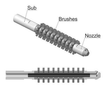
The Mechanical Brush consists of set of changeable brushes and subs for setting. For lowering on coiled tubing with downhole drilling motor the tool has watercourse and connecting tool-joint thread. Operating principle of brush is based on mechanical cleaning of inner surface of tubing and drilling pipes. The brush is inserted inside pipe with stem or DDM and is moved throughout the length. The Brush works in reciprocating motion with rotation.
